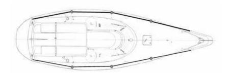
15.18.3 Pulpits, stanchions, and stanchion bases shall be constructed of stainless steel.
