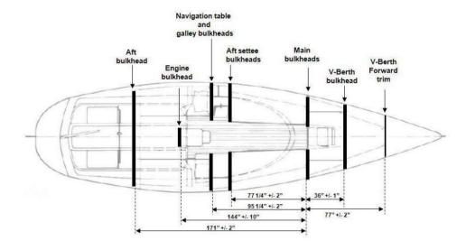
15.4.5 The main bulkheads, settee bulkheads, and the sink and chart table bulkheads, shall not be
