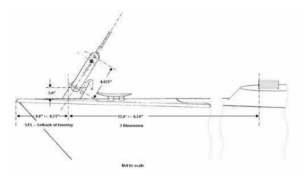
15.10.2 Vertical dimension (Measurements forthcoming) While bearing the weight of the mast and rigging alone, the upper mast bearing surface at the forward edge of the "socket" portion of the deck---mounted mast base casting shall be located a minimum of "X" inches above the top of the toe rail port/starboard of the front of the casting, measured by sighting across a string stretched across the deck "y" inches above the top of the toe rail. (Drawing 15.12.2)
