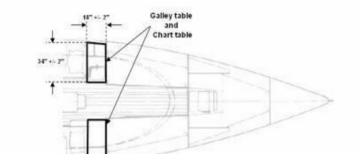
15.4.13 The deck supports connected from the galley table to the deck and the chart table to the deck may be tied positively into the deck.
