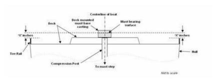
15.10.3 To meet the mast base height requirement, the mast compression post may be replaced, lengthened, shortened or permanently shimmed with durable metal shim material. When the mast base height is measured, the compression post shall be in contact with the mast base casting at the top and the load bearing structure at the bottom such that no vertical movement is possible between the two while bearing only the weight of the mast with no shroud or stay tension applied.
